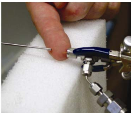
Photograph S3 Aqueous alcohol being sprayed onto outer skin surface to detect compounds including drugs and metabolites by DESI
