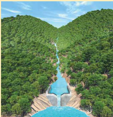
Figure 2-1 Controlled field experiment to measure the effects of deforestation on the loss of water and soil nutrients from a forest. V-notched dams were built into the impenetrable bedrock at the bottoms of several forested valleys (left) so that all water and nutrients flowing from each valley could be collected and measured for volume and mineral content. These measurements were recorded for the forested valley (left), which acted as the control site. Then all the trees in another valley (the experimental site) were cut (right) and the flows of water and soil nutrients from this experimental valley were measured for 3 years.
