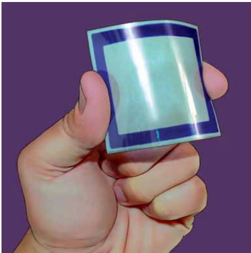
Photo 6 Flexible solar cells manufactured with use of nanotechnology
