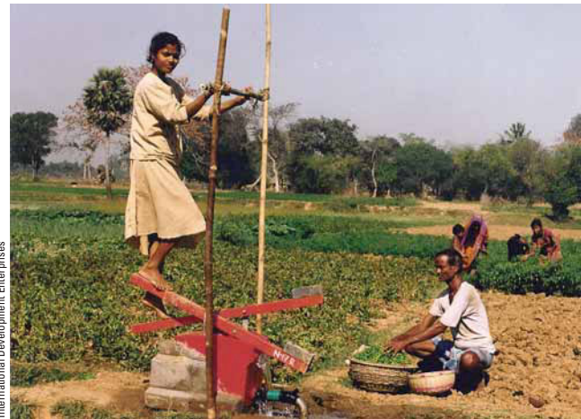
Photo 8 Treadle pump used to supply irrigation water in parts of Bangladesh and India
