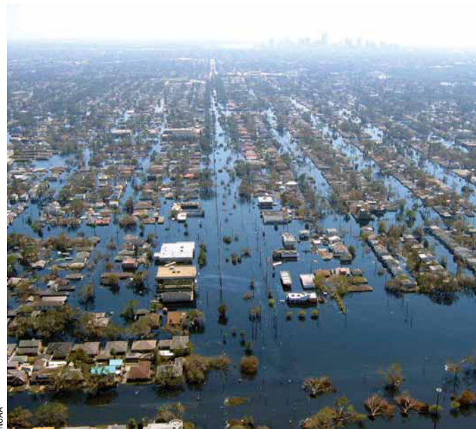
Figure 8-18 Much of the U.S. city of New Orleans, Louisiana, was flooded by the storm surge that accompanied Hurricane Katrina, which made landfall just east of the city on August 29, 2005. When the surging water rushed through the Mississippi River Gulf Outlet, a dredged waterway on the edge of the city, it breached a floodwall, and parts of New Orleans were flooded with 2 meters (6.5 feet) of water within a few minutes. Within a day, floodwaters reached a depth of 6 meters (nearly 20 feet) in some places; 80% of the city was under water at one point. The hurricane killed more than 1,800 people, and caused more than $100 billion in damages, making it the costliest and deadliest hurricane in the U.S. history. In addition, a variety of toxic chemicals from flooded industrial and hazardous waste sites, as well as oil and gasoline from more than 350,000 ruined cars and other vehicles, were released into the stagnant floodwaters. After the water receded, parts of New Orleans were covered with a thick oily sludge.
