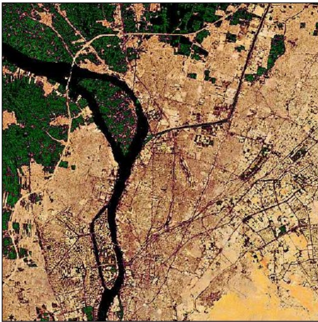
3. Combination of Landsat ETM bands 3,2,1 to form a near real colour satellite image of Cairo.
