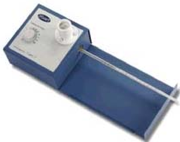
Fig. 1 Melting point device used in laboratory exercise
