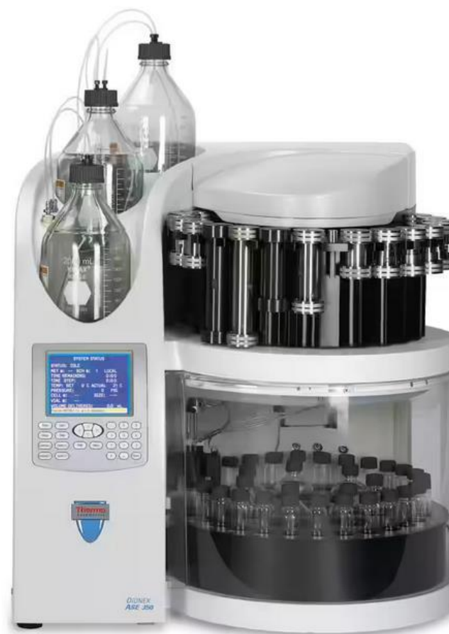
Figure 5. Scheme of an accelerated solvent extraction (ASE) system (from Richter et al. , 1996).
