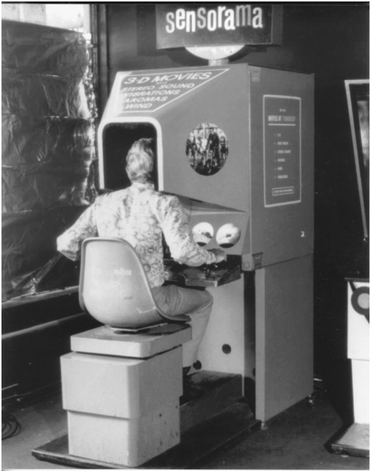
Figure 4.11 Sensorama Simulator. Inventor: Morton Heilig, 1962 < http://www.cinemedia.net/CCP/data2.htm >.
