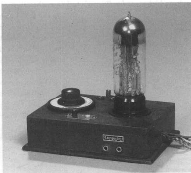
Radio receiver OE 333 with the Loewe threefold tube 3NF.
