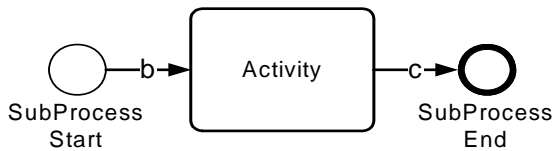
Figure 12.11 - Contents of Collapsed Sub-Process
