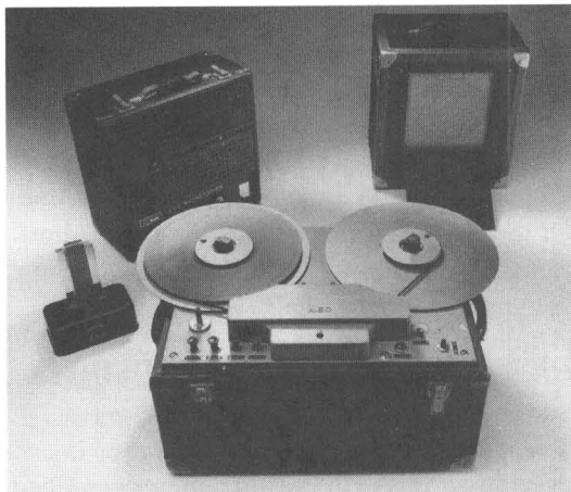
Plate 1.19 The AEG Magnetophone. (AEG)
