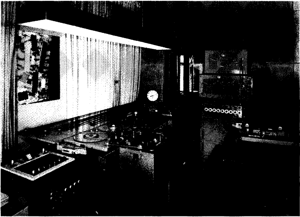
Plate 2.4 A section of the WDR Studio for Electronic Music, Cologne, in 1966, when Stockhausen was composing Hymnen . From left: corner of a four-track tape recorder; mixing console; mono tape recorder; Springer (in front of the mono tape recorder) with rotating head for suspending sounds; board with six roller guides for long tape loops; switching board with three sliding faders; sound meter; large stopwatch; second mono tape recorder; nine-octave filter; two Albis filters; portable Telefunken M5 tape recorder. (Stockhausen Verlag)
