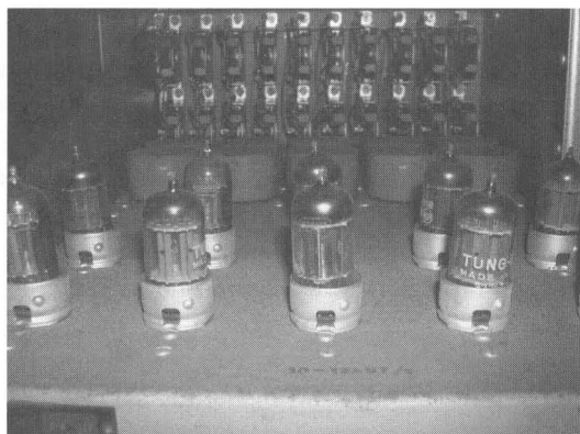
Plate 6.7 Close-up of the rear panel housing circuits and vacuum tubes for one of the “resonator” modules of the RCA Mark II. (Photo by Thom Holmes)
