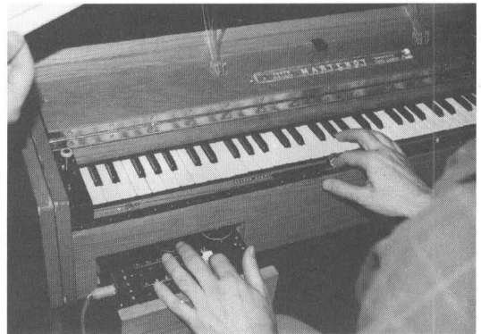
Plate 1.15 A keyboard model of the Ondes Martenot. The left hand is positioned on the expression controls. The index finger of the right hand is inserted into the finger ring. Any individual key could be jiggled laterally to produce vibrato. (Photo by Thom Holmes)
