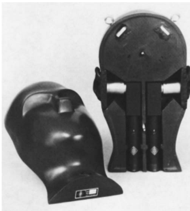
Figure D-1 A dummy head used for binaural recording (courtesy: Neumann USA).
