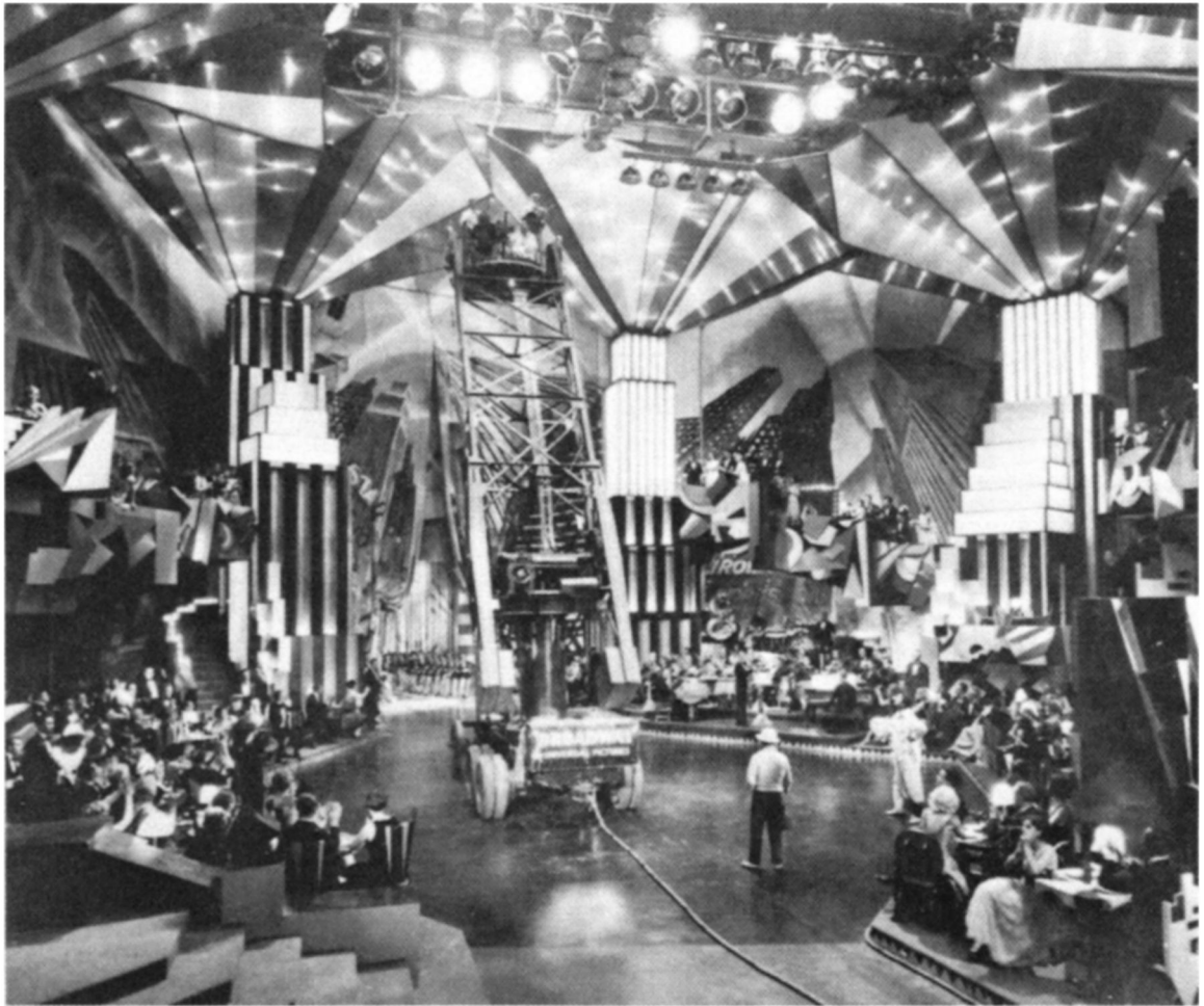
23.18 (below) The 28-ton steel crane used to film Broadway (1929). The arm was over 30 feet long
