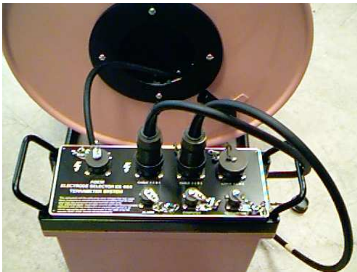
Figure 22. Connecting both ends of one LUND cable to the ES464 / ES10-64eC / ES10-64C.
