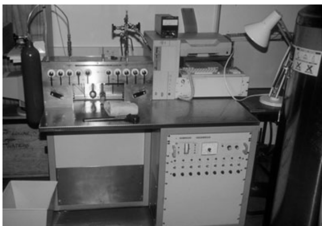
FIGURE 10-4B A venerable stable isotope ratio mass spectrometer (VG602E), which requires manual input of \text{CO}_2 and \text{N}_2 gas samples. University of Cape Town, Stable Light Isotope Laboratory. Photo by R. H. Tykot.
