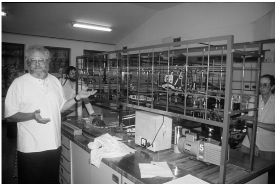
FIGURE 10-4A Off-line gas sample preparation system for stable isotope samples, with Nikolaas J. van der Merwe. University of Cape Town, Stable Light Isotope Laboratory. Photo by R. H. Tykot.
