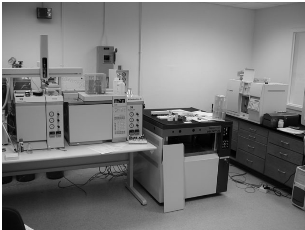
FIGURE 10-5A Example of a modern stable isotope ratio mass spectrometer (Finnigan MAT Delta Plus XL), run by computer (far right), and connected with several input devices including a Carlo Erba CHN analyzer (upper right corner) that converts organic samples into \text{CO}_2 and \text{N}_2 gas. University of South Florida, Paleolab. Photo by R. H. Tykot.
