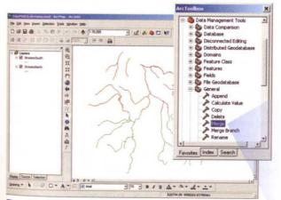
The Merge tool, located in the General toolset (Data Management toolbox) lets you combine two or more datasets of the same type into a single dataset. Specify the input datasets, and the name and location of the output dataset.
