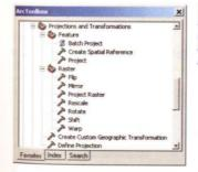
The Raster toolset under Projections and Transformations (in the Data Management toolbox) contains tools for projecting and adjusting raster datasets.
