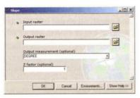
Opening the Slope tool from the Surface Toolbox opens a dialog box that prompts you for the tool parameters.
