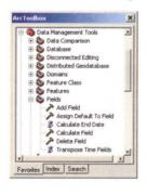
Tools for working with fields can be found in the Fields toolset, located in the Data Management toolbox.
