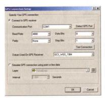
Use the GPS Connection Setup dialog box to specify the communication parameters for the GPS receiver.
