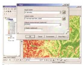
The Slope tool calculates the maximum rate of change from a cell to its neighbors, which is typically used to indicate the steepness of terrain.
