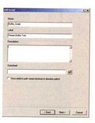
When you run the script in ArcToolbox—the same way as with any other tool—a dialog box opens that prompts the user for the input and output datasets and any parameters.
