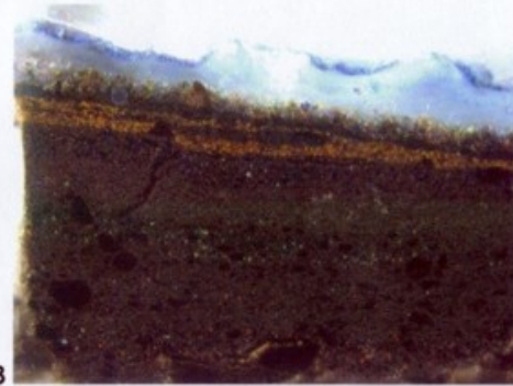
Cross-sections, visible illumination, 280x printed magnification (images overexposed to reveal black layers)
