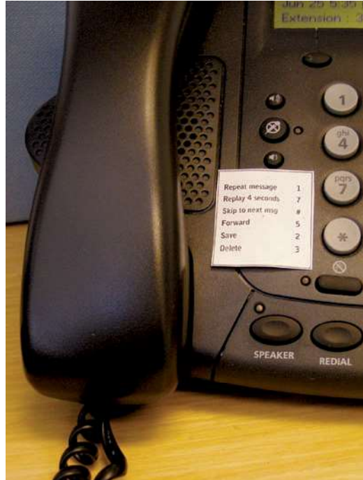
Figure 7.1. This telephone has a small cheat sheet of common voicemail commands taped to it. It probably represents an opportunity for improving the design of the system.
