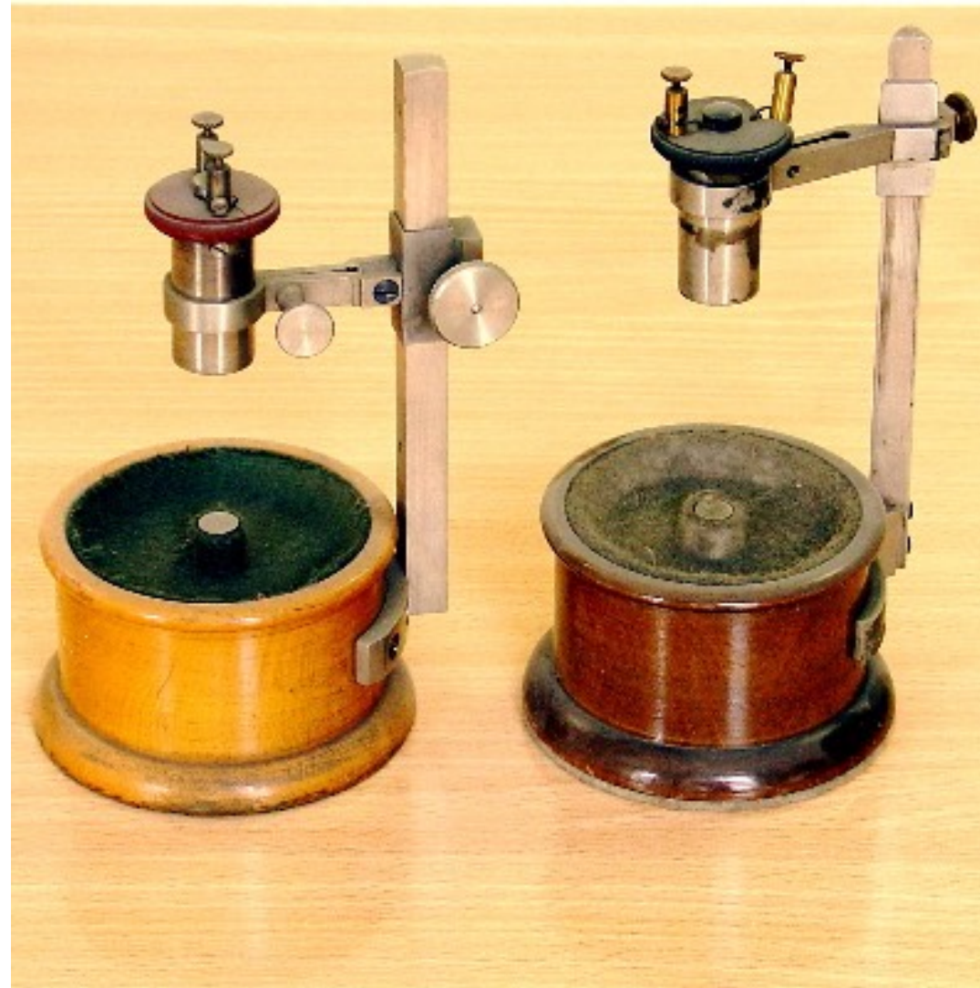
Zoth's instrument for testing acuteness of hearing
