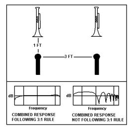
much milder cancelling and reinforcing effects when mixed with the intended microphone's signal. If, in addition, the two microphones have directional polar responses, the difference in their electrical signals will be even greater, making the Comb Filter Effect even weaker.
