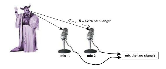
The first maximum occurs when n = 1; i.e.  $\delta = \lambda$ ; and we can work out the frequency, *f*, at which this occurs:
