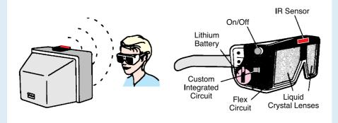
Figure 5: Alternating images on the monitor screen with alternating shutters for 3D stereo-viewing (Mike Shand)
