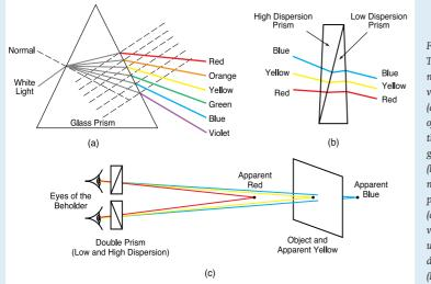
Figure 9: The basis of chromo-stereoscopic viewing. (a) The refraction of white light through a glass prism. (b) The superchromatic double prism. (c) ChromaDepth viewing spectacles using a pair of double prisms (Drawn by Mike Shand)
