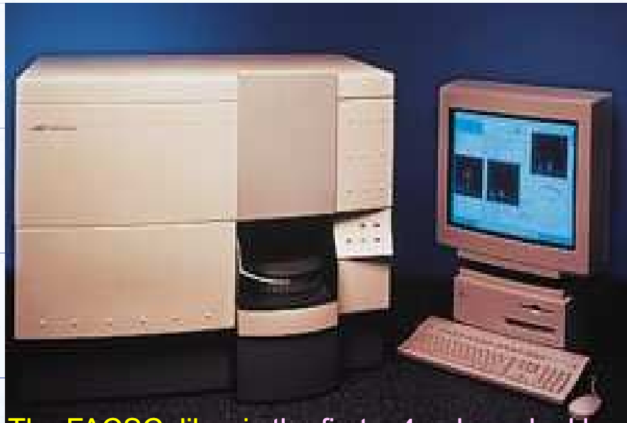
The FACSCalibur is the first a 4-colour, dual laser,
