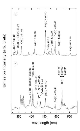
LIBS spectra from (**a**) cadmium yellow lemon (Cd0.9Zn0.1S BaSO4)Đ the asterisks indicate emission lines due to zincĐ and (**b**) chrome yellow (PbCrO4). Laser wavelength: 1064 nm.
