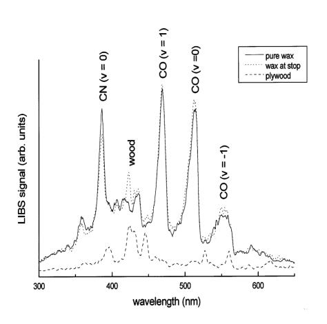
To manually remove wax from canvas or wood is time-consuming. Using a laser, it can be easily automated using LIBS-detection. The LIBS spectra from the wax show clear CO and CN bands. As soon as the underlying layer is hit, a peak appears at 423 nm. A simple selection criterion was defined in the software, telling the laser to stop firing at the moment that the peak at 423 nm emerged. LIBS spectra are shown of pure wax, plywood and the point where the laser just hits the wood.
