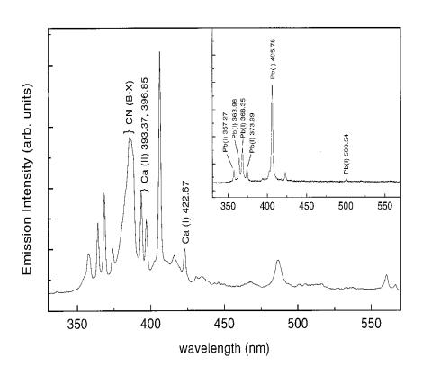
LIBS spectra of lead white oil color (lead white/linseed oil). The inset shows the spectrum of pure lead white powder. Laser wavelength: 1064 nm.
