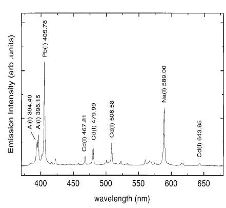
LIBS spectra from a homogenized mixture of pigments containing lead white, cadmium red, and ultramarine blue. Laser wavelength: 266 nm.
