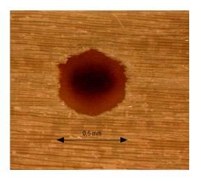
Microscope pictures of penetration hole (left) and section of the penetration channel (right) after 450 laser shots, pulse energy 55 mJ.
