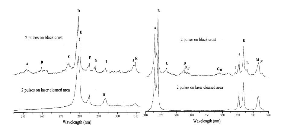
LIBS spectra in the spectral region from 245 to 310 nm obtained by two laser pulses each on the black crust and the laser-cleaned region.
