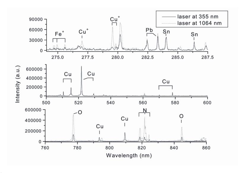
Comparison between the spectra produced by the laser at 355 nm and those produced by the laser at 1,064 nm. From top: magnifications of the UV, visible and IR spectral regions, respectively
