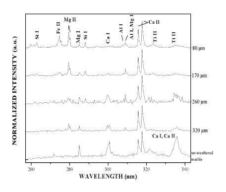
The LIBS spectra of the ablated material from a dendritic crust at different depths from the surface and un-weathered Pentelic marble, normalized to the intensity of Ca II line at 317.93 nm.
