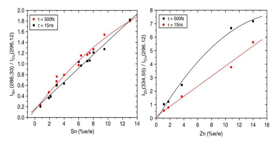
Calibration curves for Sn in all the bronze alloys studied for nanosecond and femtosecond excitation. The line of SnI at 286.33 nm was normalized with respect to the line of CuI at 296.12 nm.
