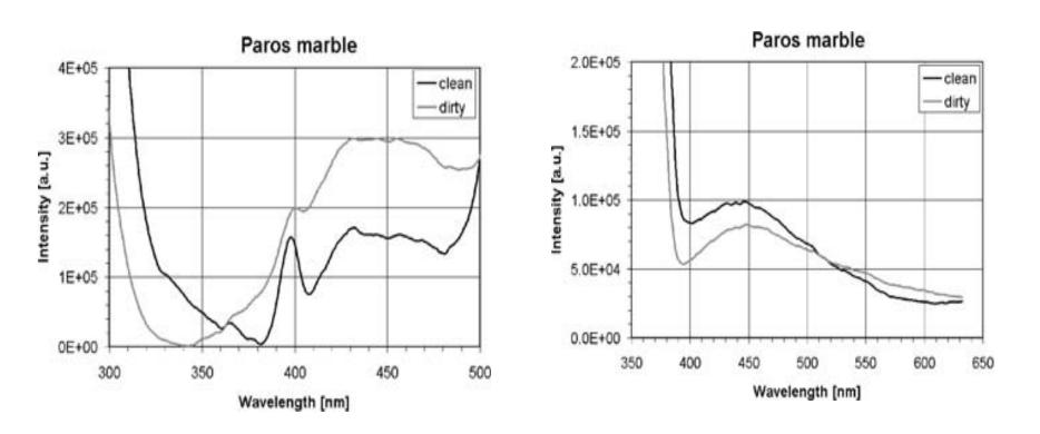
LIF spectra of Paros marble clean and encrusted surface: laser exc. at 266nm (*left*) and 355nm (*right*)
