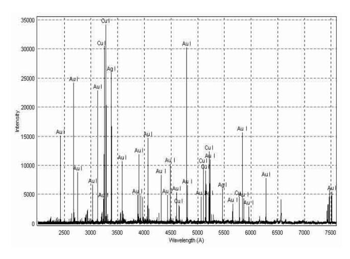
LIPS spectral signal collected during the analysis of the Au alloy. Specic lines emitted by Au, Ag and Cu atoms are marked.
