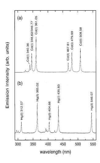
LIBS spectra from (**a**) cadmium red (CdSe0.3S0.7) and (**b**) vermillion (HgS). Laser wavelength: 1064 nm.
