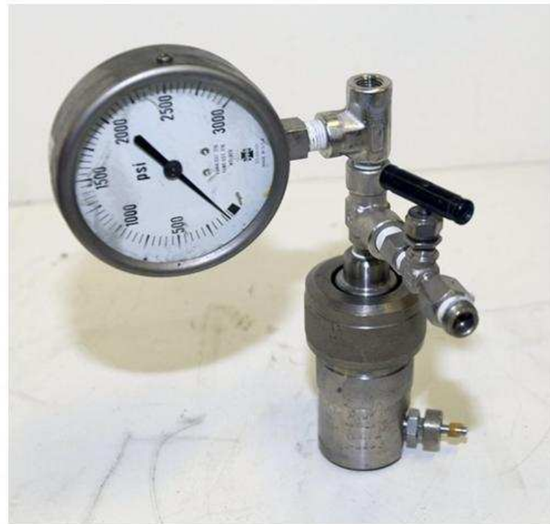
FIGURE 2.1. Nitrogen cavitation vessel. The image shown is the Parr Instrument Company Model 4639 Cell Disruption Vessel, designed specifically for small samples from 30 ml down to less than one milliliter. (Parr Instrument Company 4636 and 4639 Cell Disruption Vessels.)
