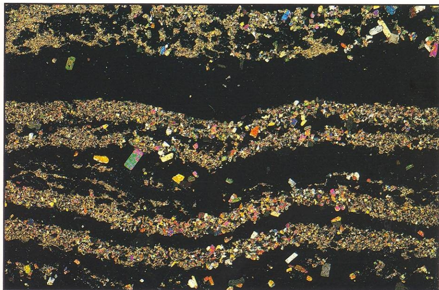
138 Halite and anhydrite with crossed polars. Locality: Permian, northeast England (x 12).
