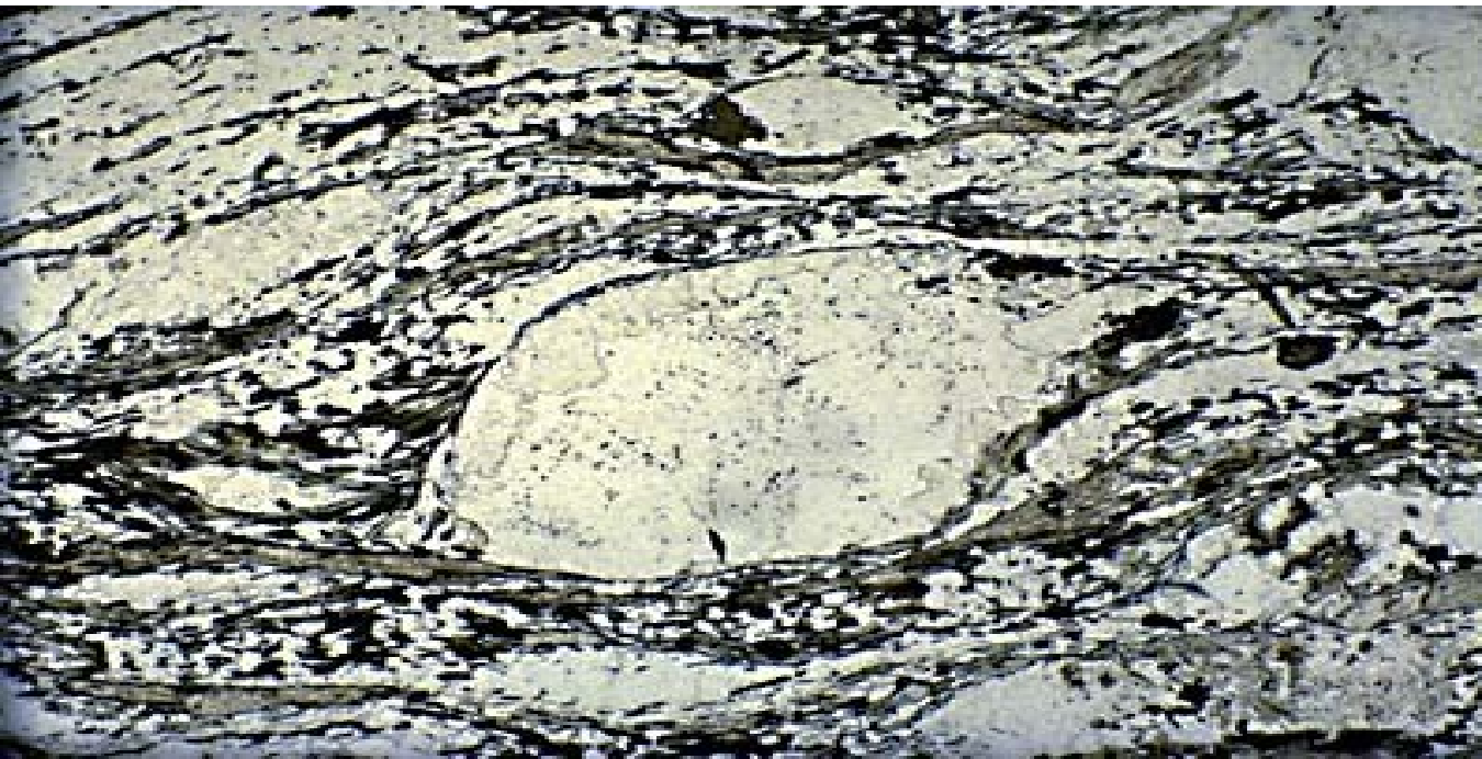
Mica fish: Sheared porphyroblasts of biotite in a quartz mica schist. Note the presence of tourmaline crystals (Tm), and the pressure fringes of quartz around the biotite porphyroblast.
