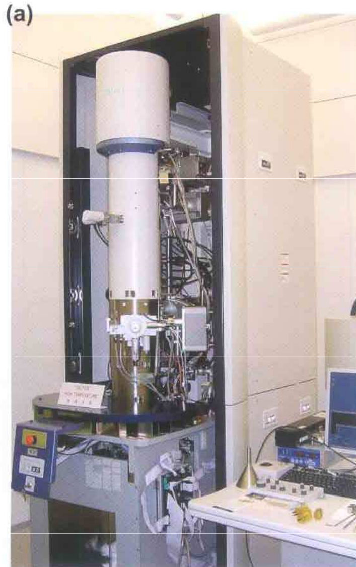
Fig.1(a) The Hitachi aberration corrected HD2700C STEM at BNL. (b) The schematics of the lens and detector assignment of the instrument.
