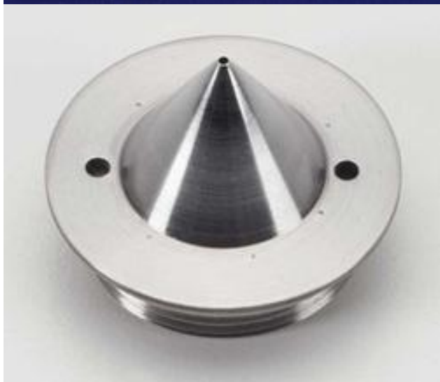
Obr. 9 Apertury rozhraní: Sampling cone a Skimmer cone .
