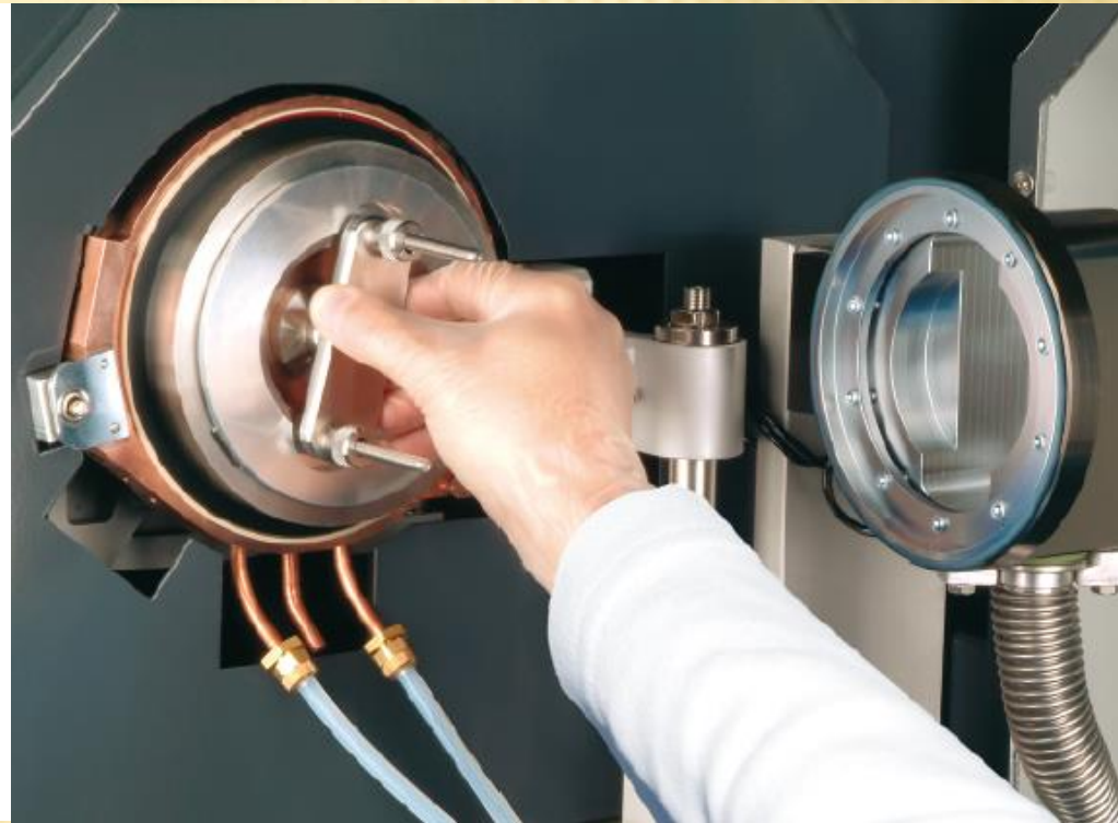
Placement of the sample holder in the GD ion source
