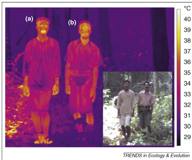
Figure 2. Thermographic image of Batek hunter-gatherers after a 1 h hike in their rainforest habitat (Taman Negara National Park, Malaysia). Internal and external body temperatures can be estimated using a thermographic camera. Analysis of pixels from the open mouth provides a good estimate of core body temperature. The open-mouth pixels of the taller man (a) (~164 cm) show an elevated core temperature of 38.0 °C, whereas those of the shorter man (b) (~156 cm) show a normal core temperature of 36.9 °C. An estimate of the skin surface temperature based on facial pixels excluding the open mouth did not differ substantially between them (mean values of 36.1 °C and 36.4 °C, respectively). Although not representing a formal test of the thermoregulatory hypothesis as an explanation for pygmy phenotype evolution, the higher core body temperature of the taller man following physical activity illustrates the plausibility of its underlying premise—that in tropical rainforests, where the thermoregulatory mechanism of sweat production and evaporation is inefficient, smaller bodies might confer a fitness advantage by generating less internal heat during activity. Images were captured with a ThermoCAM SC640 (FLIR Systems, Boston, MA, USA) under photographic license number 395108 issued by the Department of Wildlife and National Parks, Malaysia.
