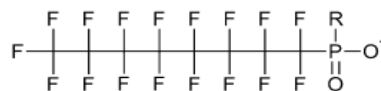
Perfluorophosphonic/phosphinic acids (ex. If R=OH then PFOPA If R=C8 perfluoroalkane then 8:8 PFPI)
