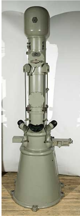
First commercial EM, 1937 Metropolitan-Vickers EM1 (EM2 shown)
