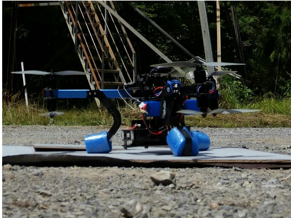
3DRobotics Y6 hexacopter outfitted with a gimbal-mounted Canon Powershot S110 compact camera
