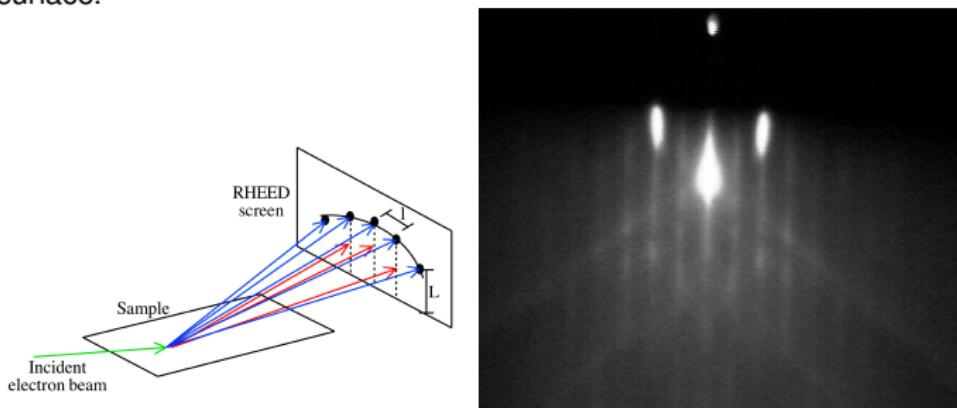
Figure shows a typical pattern on the screen for electrons reflected from a smooth surface, in which constructive interference between some of the electrons reflected from the lattice structure results in lines. If the surface is rough, spots will appear on the screen, also.
