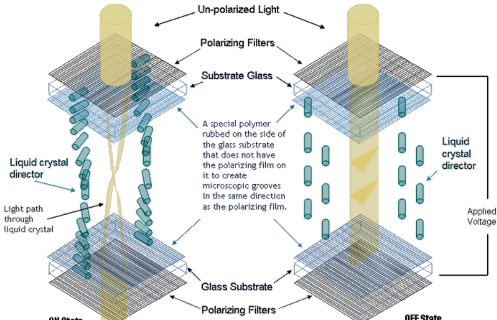
Cross-Sectional View of an LCD Panel
