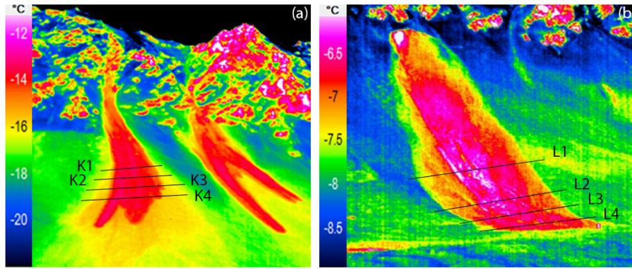
**Figure 6.** IRT camera images for avalanches (a) #1a and #1b and (b) #2. Note the different temperature scales amongst the avalanches. Black lines indicate positions of lateral snow temperature transects.
