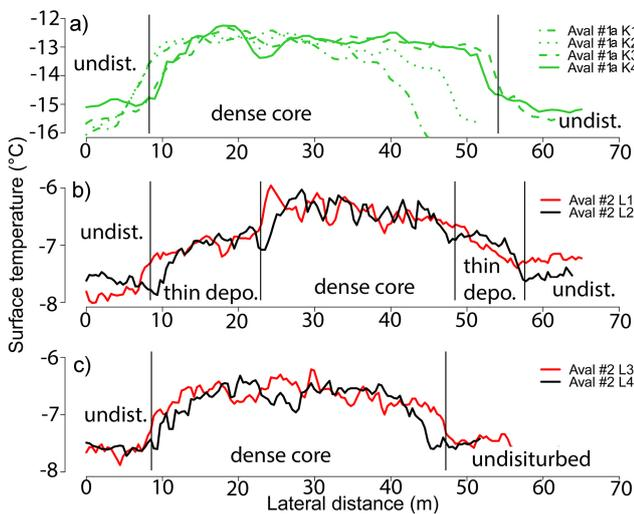
**Figure 7.** Snow surface temperatures acquired with IRT along lateral transects for avalanche #1 (a) and in the path (b) and the deposition area (c) of avalanche #2. Extent of undisturbed snow cover, thin-deposit and dense core are indicated. The lateral distance was calculated by referencing and scaling with the measured width of the avalanche.
