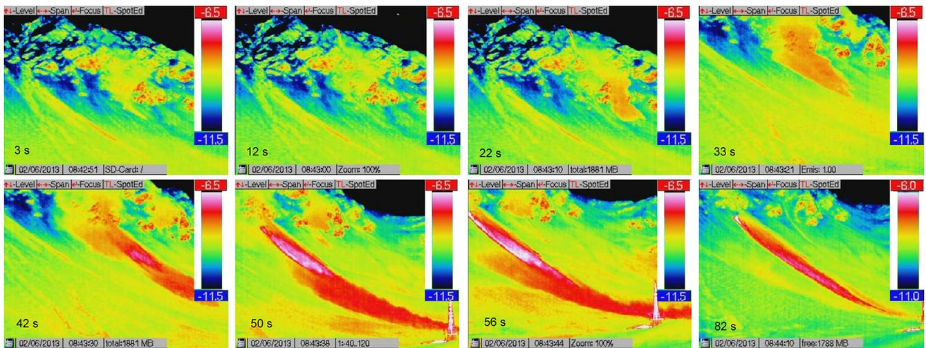
**Figure 5.** Screenshot of IRT camera videos for avalanche #2. The first picture was taken 3 s after the avalanche released. Note that the temperature scale was changed by 0.5 °C for the last shown image (82 s).
