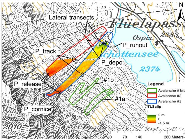
**Figure 2.** Flüelapass field site close to Davos (Switzerland). Outlines of avalanche #1a and #1b (green), #2 (red) and #3 (blue). The colour bar shows differences between terrestrial laser scans before and after the individual avalanches.  $P_{\text{release}}$  and  $P_{\text{track}}$  indicate locations of snow profile in the release and along the path, respectively. Red and blue lines indicate positions of lateral investigations and deposition snow profile  $P_{\text{depo}}$ .
