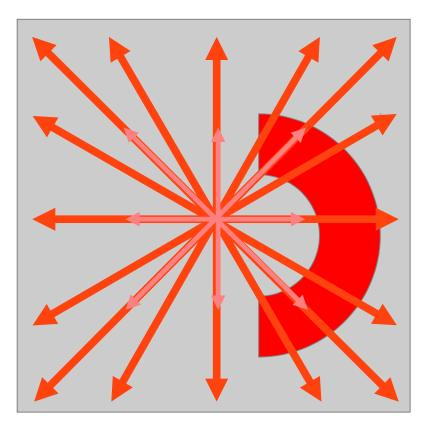
Set of all shifts of up to 1 pixel Set of all new shifts of up to 2 pixels Shifts of (0, +/-1, +/-2) pixels results in 25 orientation searches.
