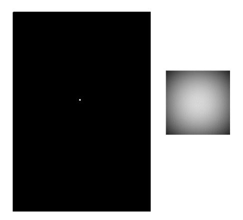
If the point was infinitely sharp, the FFT would be flat.
