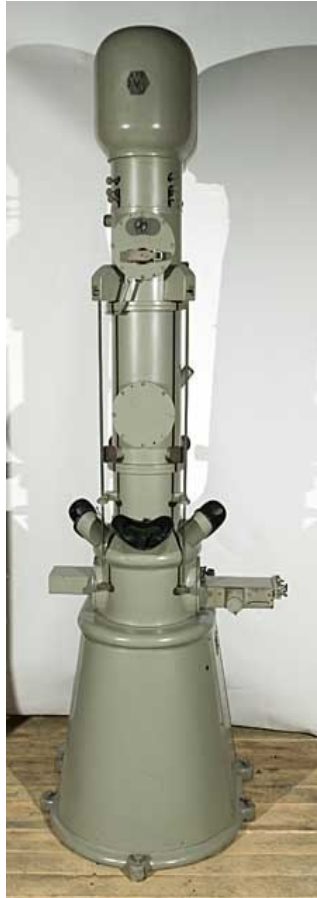
First commercial EM ( 1937 ) was Metropolitan-Vickers EM1 (EM2 shown)
