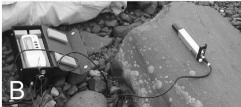
Text-fig. 3. Measuring rock surface micro-roughness of glacially-abraded boulder (A); Handysurf E35-B profilometer (B). Phot. A.Tittenbrun
