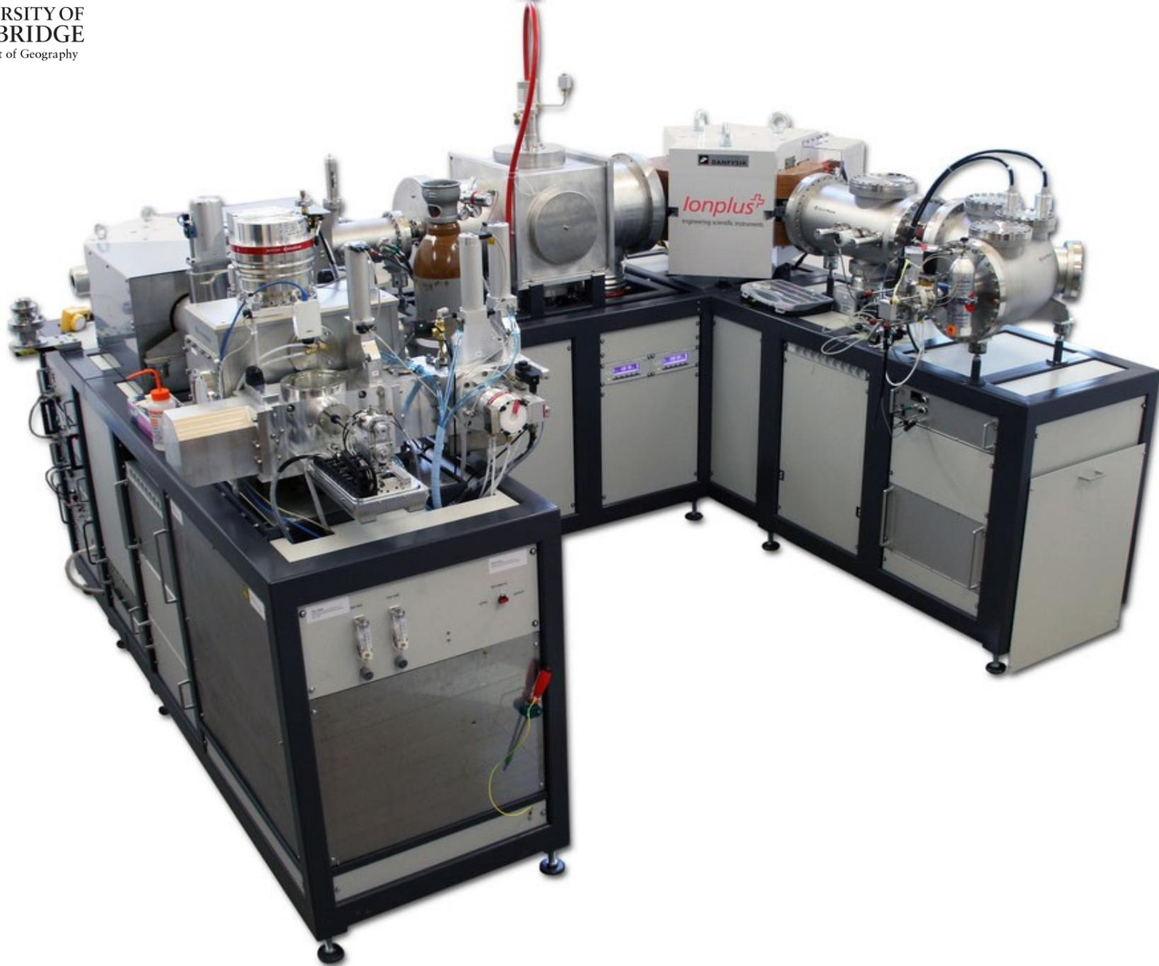
**MICADAS** - Mini Carbon Dating System (<https://www.ionplus.ch/products/micadas/>)
