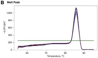
**Fig. 2.** Validation of qPCR primers. (A) qPCR is performed at a range of annealing temperatures using a thermal gradient block. Amplification profiles indicate that the most efficient amplification occurs at the four lowest annealing temperatures between 53 °C and 57.7 °C where the curves are at the lowest  $C_q$ ; (B) a single peak on the melt curve analysis indicates a single PCR product.
