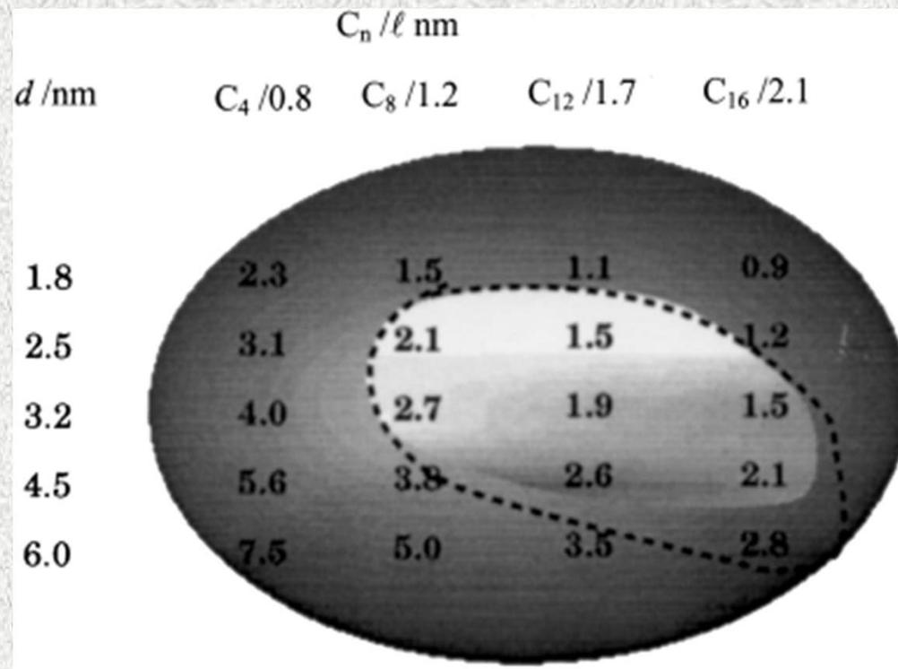
The  $d$ - $l$  phase diagram for Pd nanocrystals thiolized with different alkane thiols.
