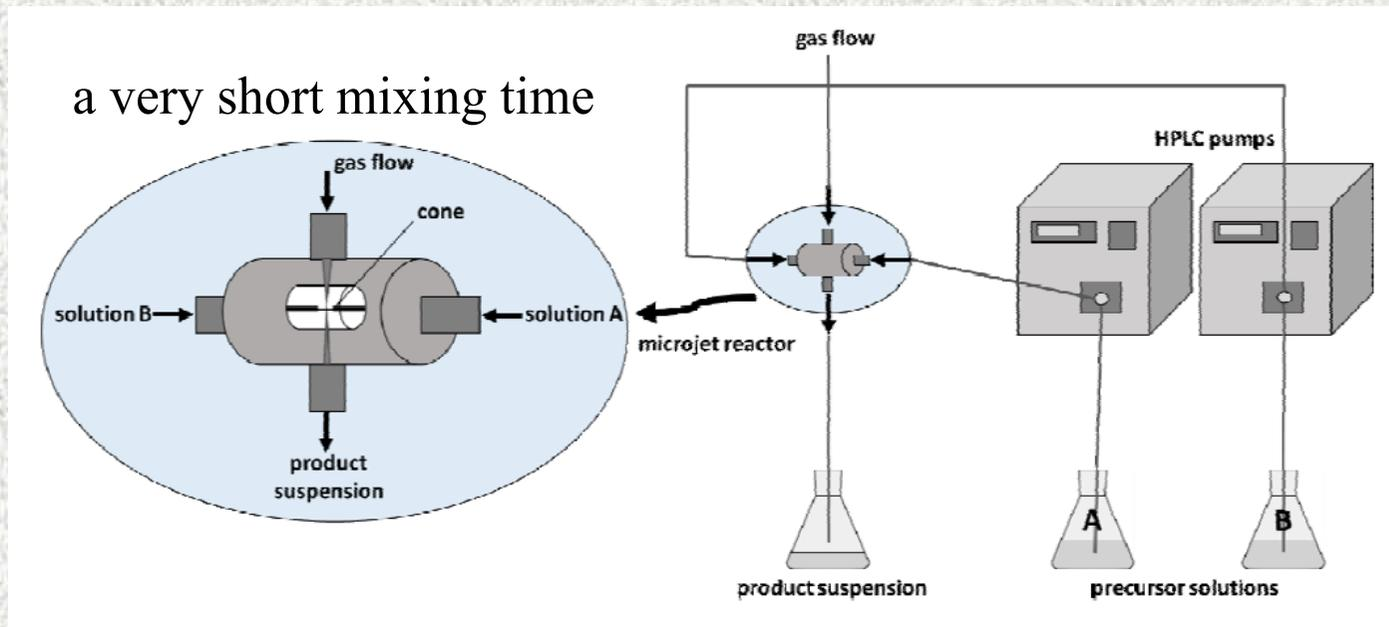
transport from the reactor to a tubing for the particle growth, the length of tubing up to the collection vessel influences the particle growth
