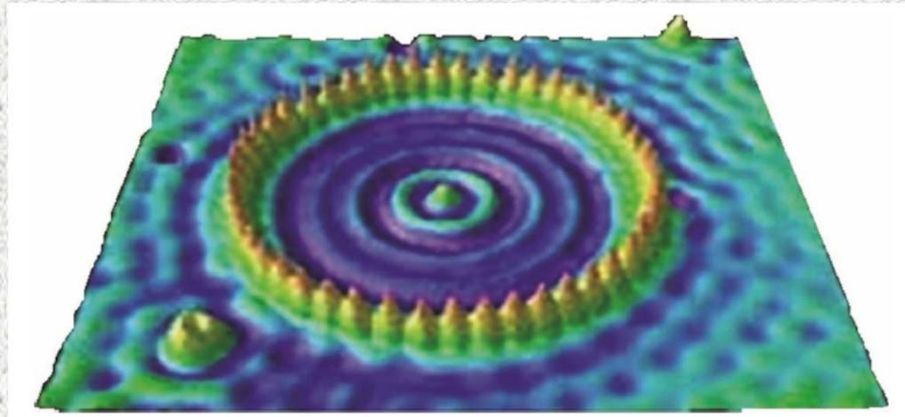
Atoms arranged on a surface form a corral confining their valence electrons. The probability density image determined by the wave function distribution captured by STM - wave function leakage into a positively biased scanning probe
