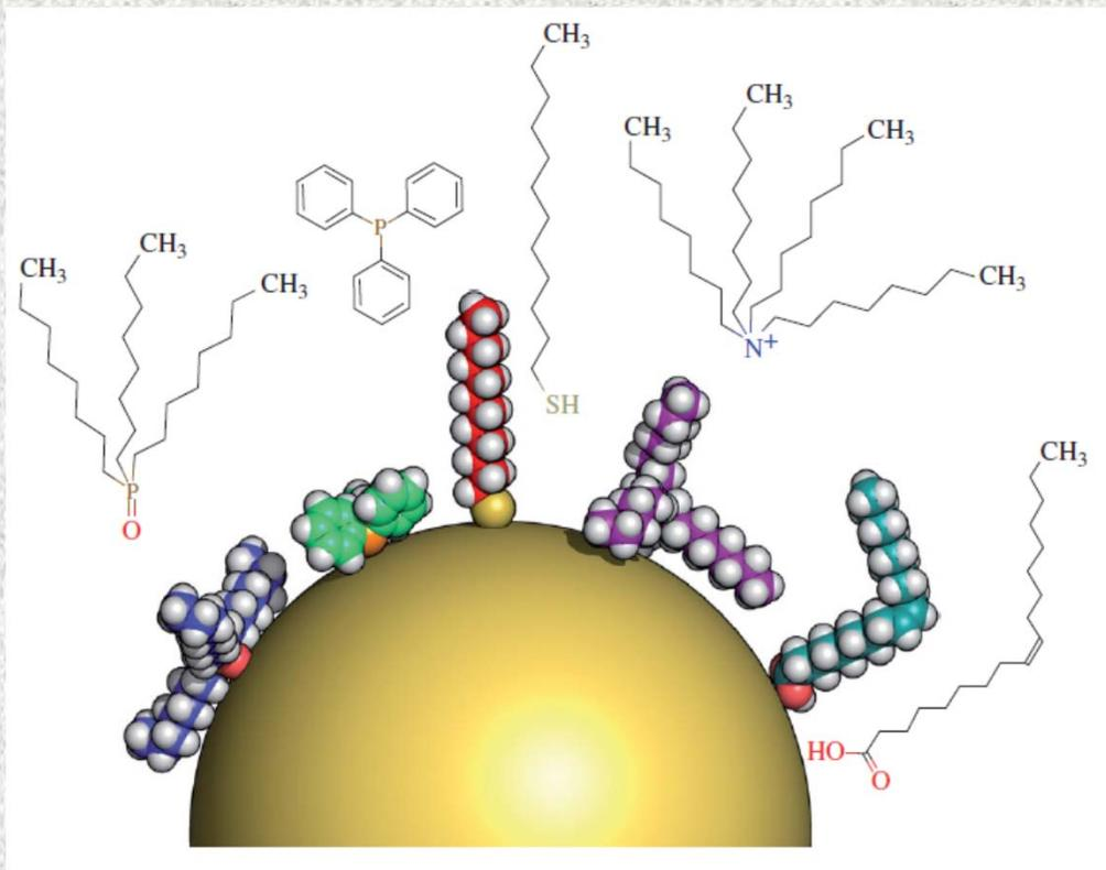
A nanoparticle of 5 nm core diameter with different hydrophobic ligands
