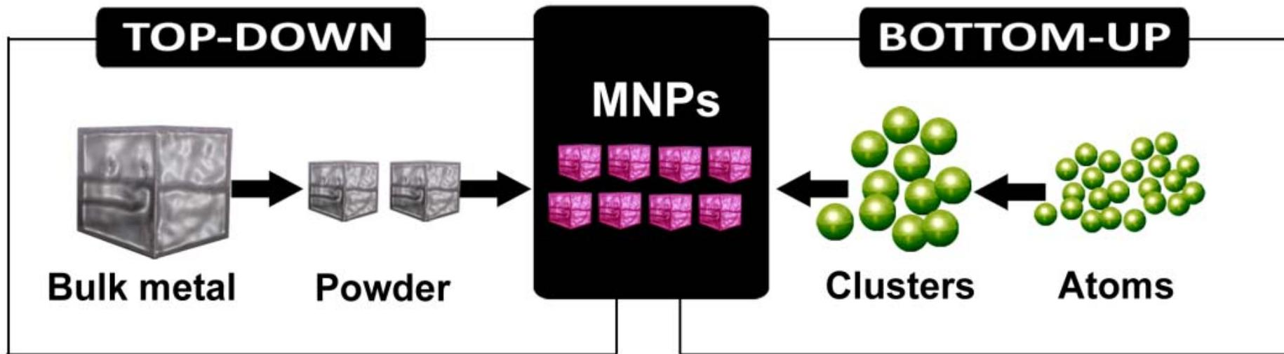
**Top-down:** from bulk to nanoparticles
