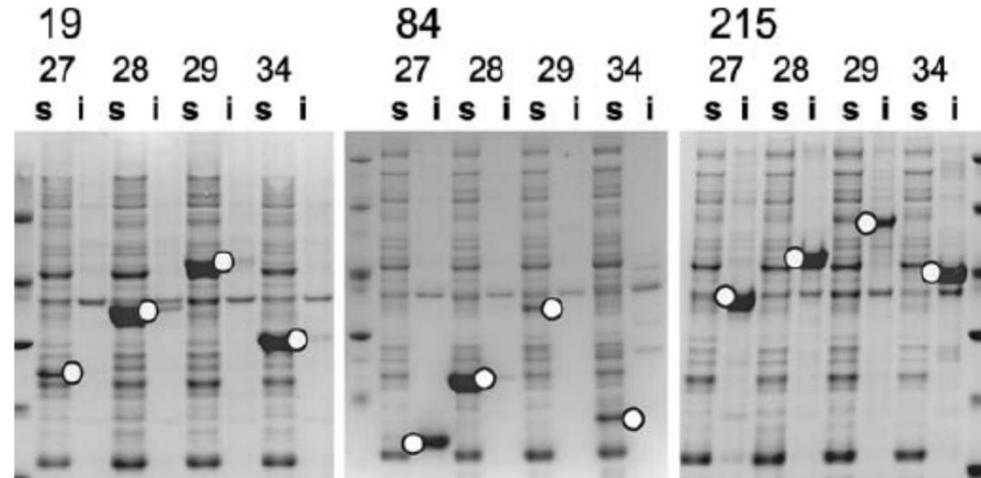
Example of SDS PAGE with **soluble (s) and insoluble (i) fractions** following lysis. The results produced from the four different expression vectors (**27: His tag only; 28: thioredoxin + His tag; 29: GST + His tag; 34: GB1 + His tag**) are shown for three different target proteins (*Hammarstrom et al., 2006*).
