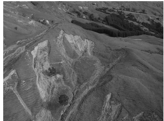
FIGURE 18.4. Multiple occurrence regional landslide event. These phenomena can occur almost anywhere in New Zealand hill country, depending on intensity and location of storm rainfall. Gisborne, New Zealand, 2002. (Photo: Michael Crozier.)
