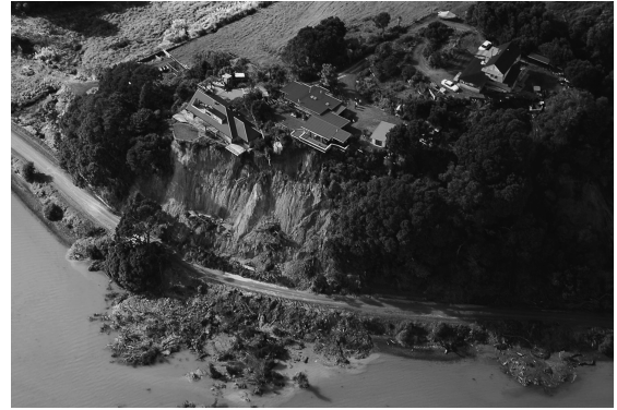
FIGURE 18.3. Former sea cliff still actively adjusting by landsliding, Orewa, New Zealand, 2006. (Photo: Graham Hancox.)
