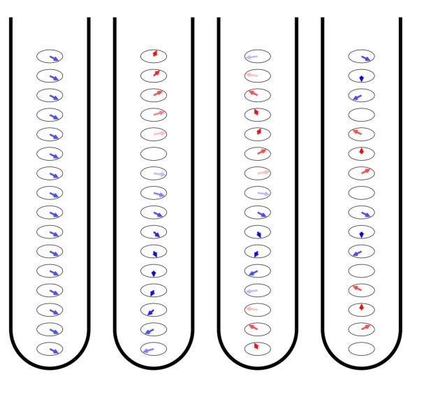
$$\gamma G_{z} z = \Omega : \qquad \langle M_{+} \rangle = K \left\langle e^{-R_{2}t} \right\rangle \mathcal{N}(z) \left\langle e^{i(0)t} \right\rangle$$
