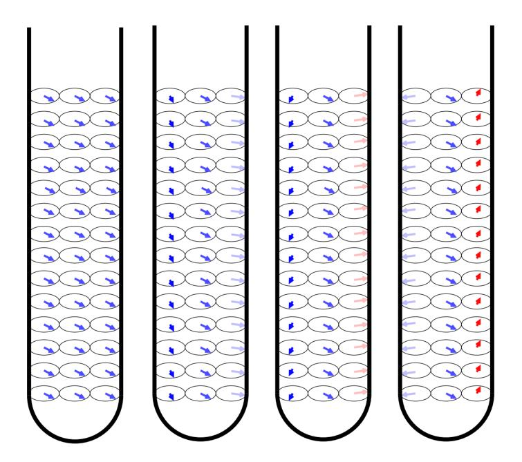
$G_{y} = \Delta B_{0} / \Delta y \quad \Rightarrow \quad \Omega'(y) = \Omega - \gamma G_{y} y$  $-\mathscr{I}_{y} \rightarrow -\mathscr{I}_{y} \cos(\Omega' t) + \mathscr{I}_{x} \sin(\Omega' t)$  $= -\mathscr{I}_{y} \cos(\Omega - \gamma G_{y} y t) + \mathscr{I}_{x} \sin(\Omega - \gamma G_{y} y t)$
