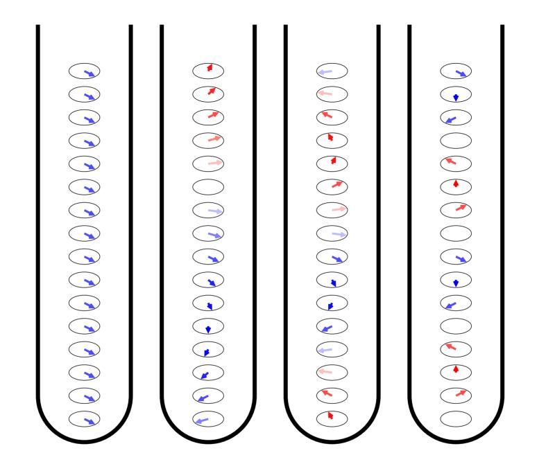
$G_{z} = \Delta B_{0} / \Delta z \quad \Rightarrow \quad \Omega'(z) = \Omega - \gamma G_{z} z$  $-\mathscr{I}_{y} \rightarrow -\mathscr{I}_{y} \cos(\Omega' t) + \mathscr{I}_{x} \sin(\Omega' t)$  $= -\mathscr{I}_{y} \cos(\Omega - \gamma G_{z} z t) + \mathscr{I}_{x} \sin(\Omega - \gamma G_{z} z t)$
