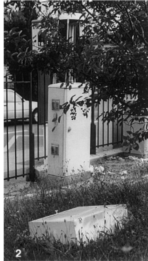
Fig. 2. Cage placed on grass in Besançon Botanical Gardens a few feet away from the device used to monitor the atmospheric lead concentration by the side of a busy road.
