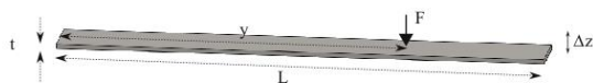
Figure 8.5: A cantilever of length L and thickness t is loaded at a distance y from the clamped end with load F , the corresponding deflection is \Delta z .
