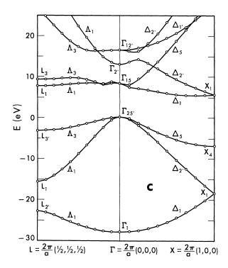
FIG. 1. The electronic band structure of diamond.
