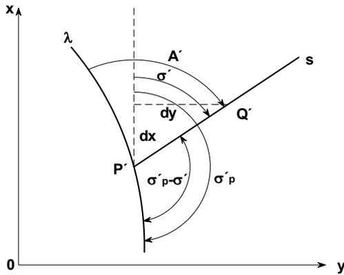
$$\operatorname{tg} \sigma' = \frac{dy}{dx} \qquad \operatorname{tg} \sigma' = \frac{\frac{\partial y}{\partial \varphi} d\varphi + \frac{\partial y}{\partial \lambda} d\lambda}{\frac{\partial x}{\partial \varphi} d\varphi + \frac{\partial x}{\partial \lambda} d\lambda}$$
