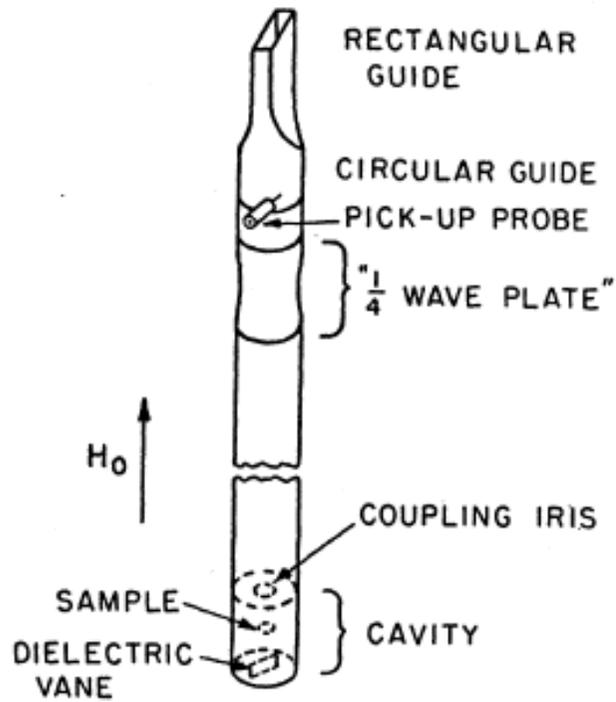
Experimental setup for measurements with circularly polarized microwave field; from Dresselhaus, Kip, Kittel, Phys. Rev. 1955.
