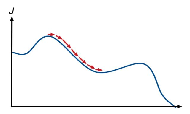
Gradient Descent is an iterative method used to find the minima of a function.
